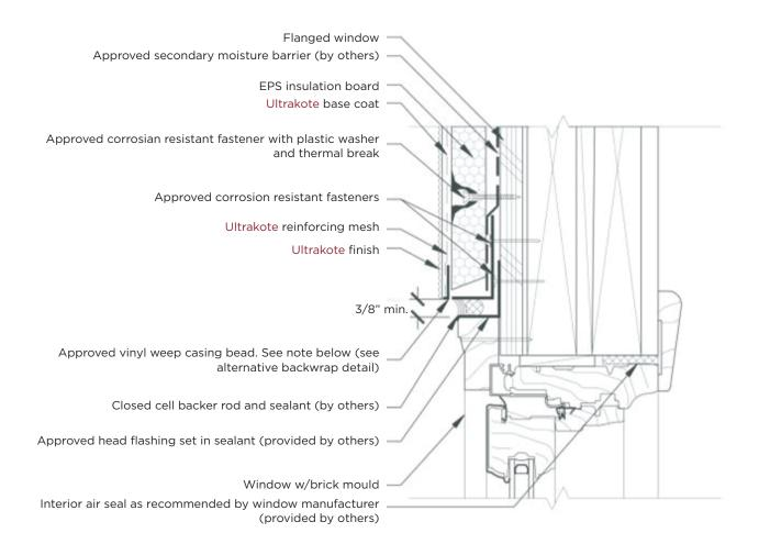
NOTE: Maintain 1/8" space between beveled insulation and weep casing bead.
